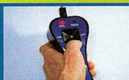
A red LED flash confirms an electrical problem with the wire harness or associated electrical system.
