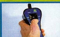
A green LED flash indicates that the wire harness and associated electrical system are functioning properly.
